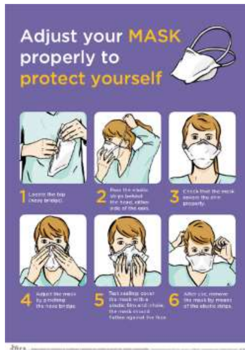
Figure 10 — Example of poster describing how to put the mask in place and check on sealing (INRS: http://www.inrs.fr/media.html?refINRS=A%20759 )
